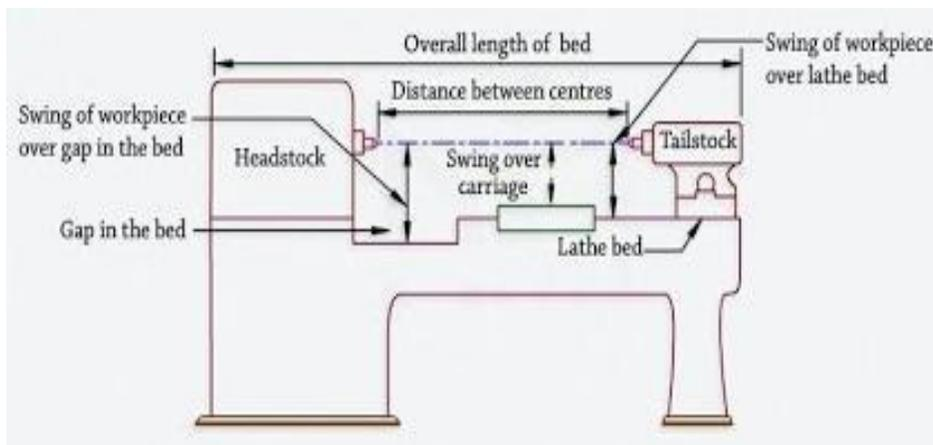
**Specification of a lathe machine**
