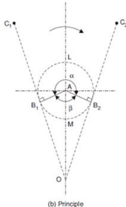
Quick return mechanism of a shaper machine
