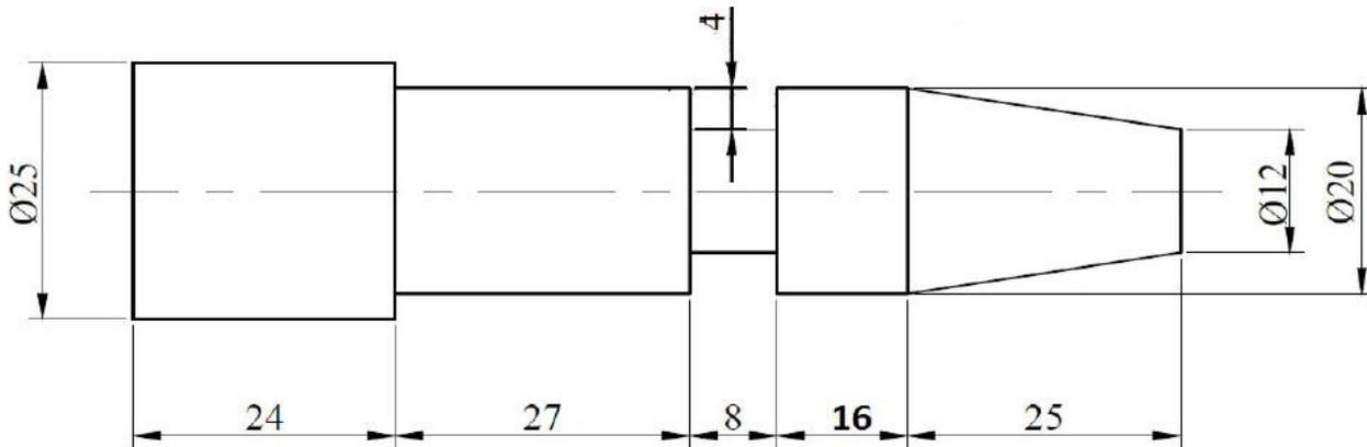
**Materials used:** Mild steel rod of  $\text{Ø } 25 \text{ mm} \times 100 \text{ mm}$
