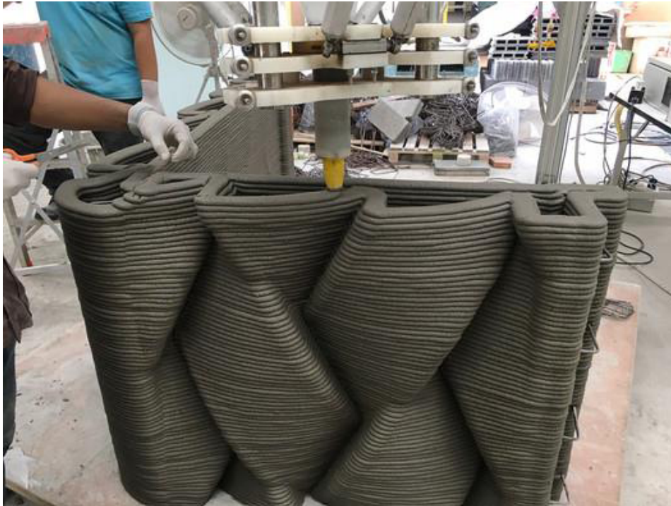
Complex structures can be printed layer by layer using specially designed concrete mixes Source: The Comeback of Craftmanship and Artisanal Aesthetics in 3D Printing | ArchDaily
